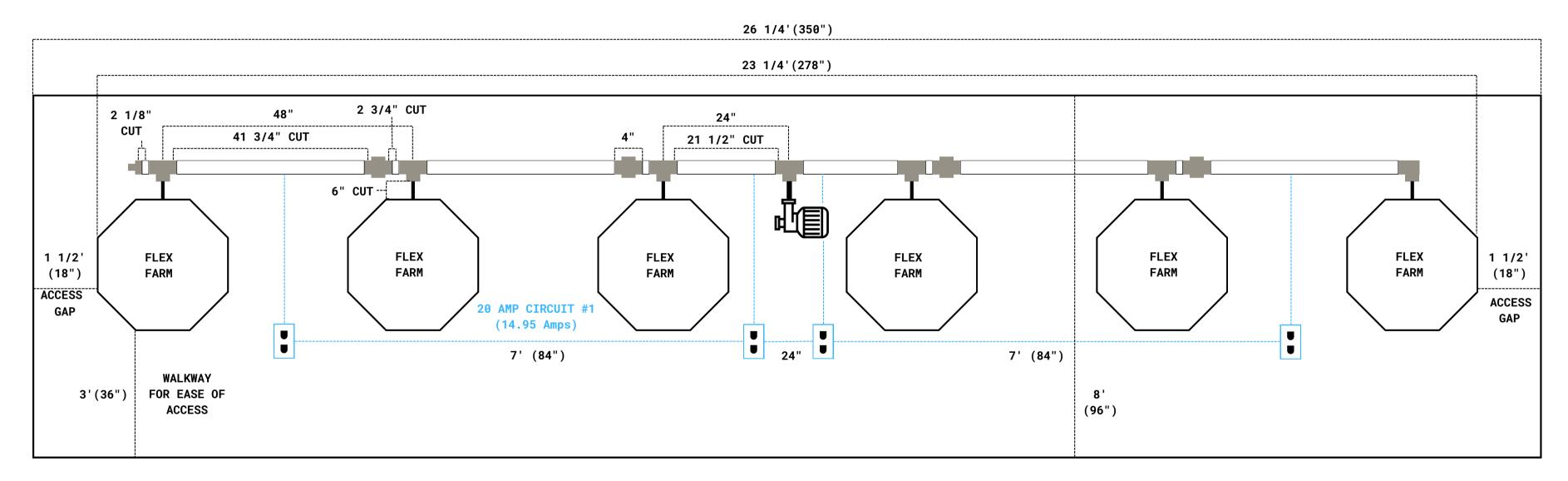
**\*ALL OUTLETS ARE SINGLE SIDED UNLESS OTHERWISE NOTED\*** \*ELECTRICAL LAYOUT CAN BE IMPLEMENTED USING WALL MOUNTED OR HANGING RECEPTACLES\*
