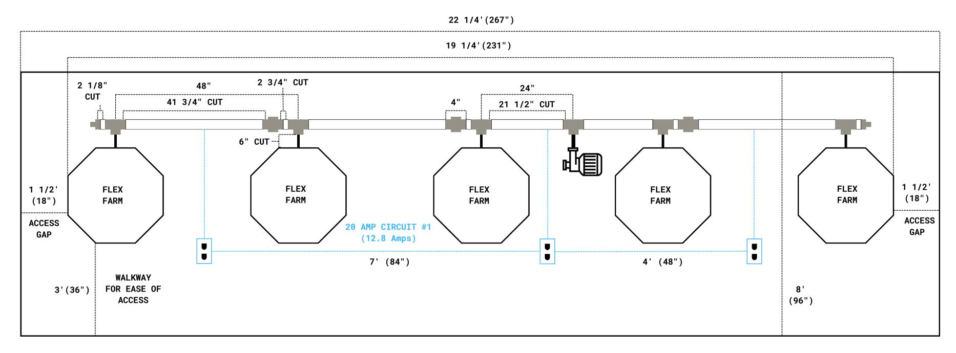
**\*ALL OUTLETS ARE SINGLE SIDED UNLESS OTHERWISE NOTED\*** \*ELECTRICAL LAYOUT CAN BE IMPLEMENTED USING WALL MOUNTED OR HANGING RECEPTACLES\*
