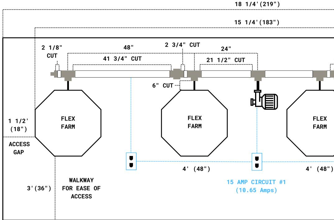
**\*ALL OUTLETS ARE SINGLE SIDED UNLESS OTHERWISE NOTED\*** \*ELECTRICAL LAYOUT CAN BE IMPLEMENTED USING WALL MOUNTED OR HANGING RECEPTACLES\*
